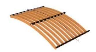
Step 3 : Panel ready to be fitted, after drilling the counter-slats for the hangers (Ø 9 mm)
