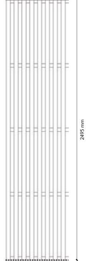
$^{\ast}$  Overhang counter-slats must always be positionned on the same side.
