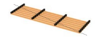
Step 3 : Screw on the profile to hold the slats
