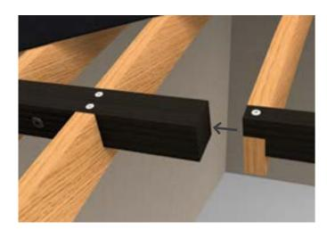
Step 3 : Fix the last panel using the joining kit
