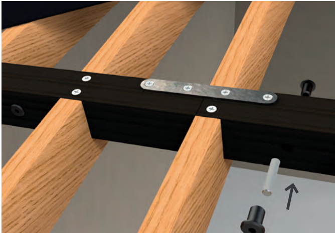
Step 3 : Fix the last panel using the joining kit
