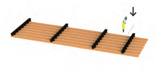
Step 4 : Screw the counter-slat back on
