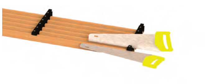
Step 5 : Notch the end of the counter-slat
