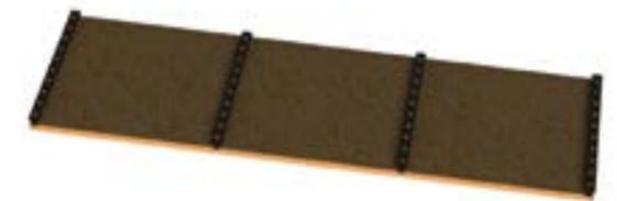
Step 3 : Fix the particle plate on the slats and draw the outline
