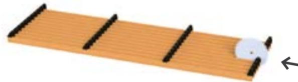
Step 3 : Male cut finish - Screw on the edging strip (option) - Pre-drill Ø 2 mm
