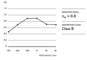
Rear side: rigid acoustic mineral wool tile 2.4 kg/m² with fleece facing (thickness: 20 mm) Not supplied by Laudescher
