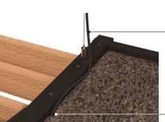
Insert the fixing part into the luminaire profile.
