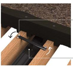
**Step 2:**Install the fixing part on top of the slats, secured by screwing
